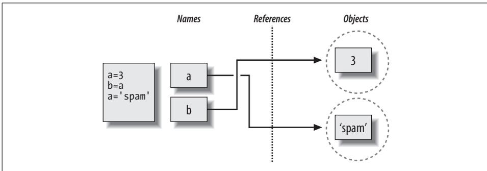
Figure 6-3. Names and objects, after finally running assignment `a = 'spam'`. Variable `a` references the new object (i.e., piece of memory) created by running literal expression 'spam', but variable `b` still refers to the original object 3. Because this assignment is not an in-place change to object 3, it only changes variable `a`, not `b`.
