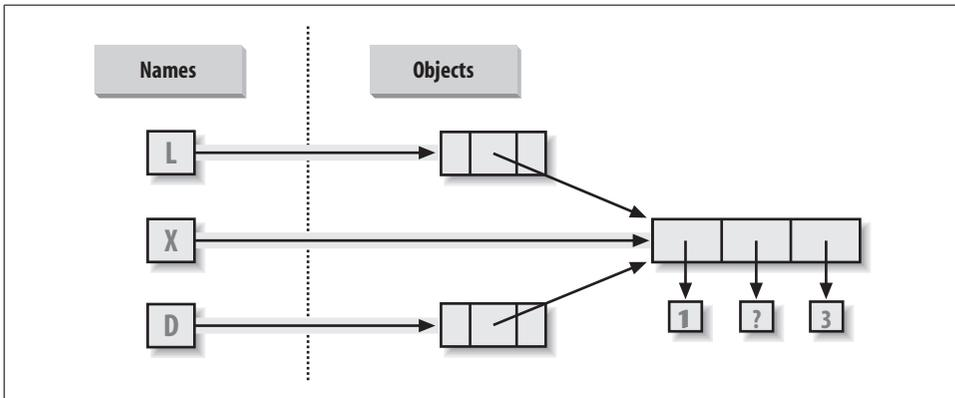
Figure 9-2. Shared object references: because the list referenced by variable `X` is also referenced from within the objects referenced by `L` and `D`, changing the shared list from `X` makes it look different from `L` and `D`, too.
