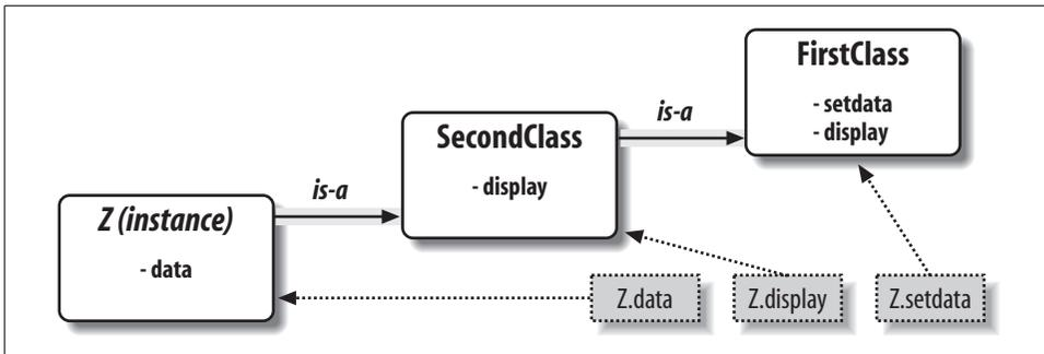
Figure 23-2. Specialization by overriding inherited names by redefining them in extensions lower in the class tree. Here, *SecondClass* redefines and so customizes the “display” method for its instances.
