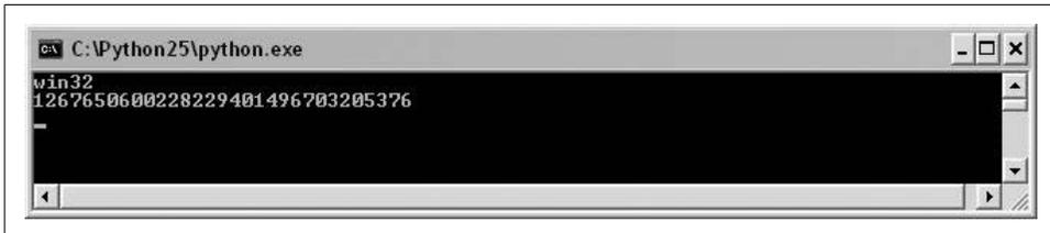
Figure 3-2. When you click a program’s icon on Windows, you will be able to see its printed output if you add a `raw_input()` call to the very end of the script. But you only need to do so in this context!
