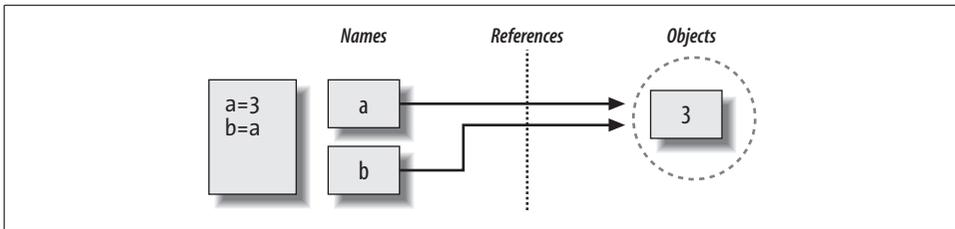
Figure 6-2. Names and objects, after next running the assignment `b = a`. Variable `a` becomes a reference to object 3. Internally, the variable is really a pointer to the object’s memory space created by running literal expression 3.
