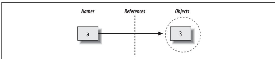
Figure 6-1. Names and objects, after running the assignment `a = 3`. Variable `a` becomes a reference to object 3. Internally, the variable is really a pointer to the object's memory space created by running literal expression 3.
